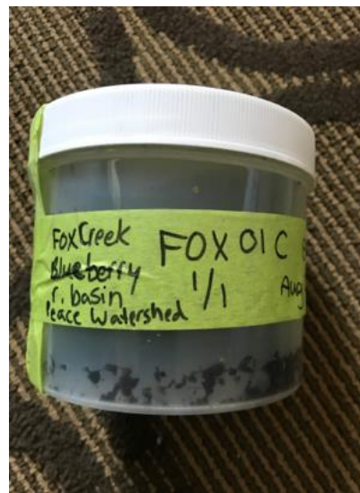
Figure 2: Correctly sealed sample
